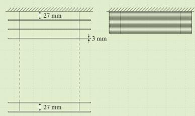
When the blind is up, all the slats are stacked at the top with no gaps, as shown in the second diagram.
